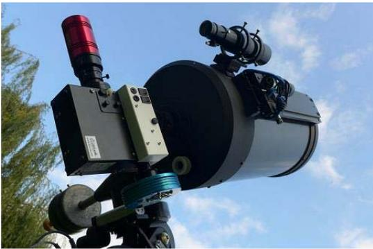
*Image : LISA spectrograph mounted on a C11*
